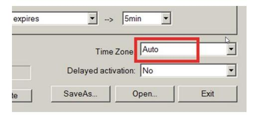
When the "Auto" time zone option is selected, then the Televend box tries to determine the time zone using data from the modem or TZ + /TZ- special handling.
