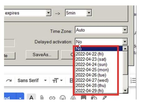
Limitation: only one configuration string with delay can be saved in Televend. If multiple configuration strings with a delay are sent to the Televend, it will only remember the last one which was sent to it.
