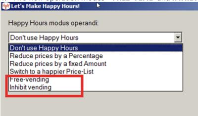
These two new Happy hour modes allow the machine to switch to the free-vend mode at a particular time or to ban sales.
